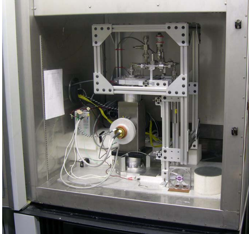
Figure 3-10: Vertical \text{UF}_6 source in the environmental chamber. This source has an enrichment of 3.3%. The active AEM used for temperature and pressure sensitivity tests is mounted on the pipe. A heat sink around the x-ray tube is visible.
